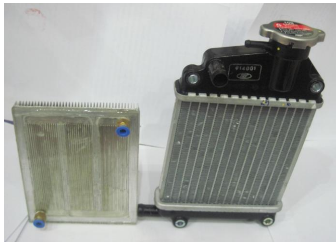
Fig. 4. Comparison between the minichannel heat exchanger and scooter radiator
